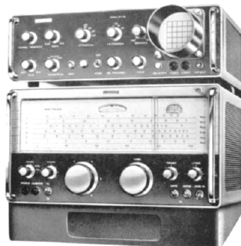
The EPR26 'Panoramic Receiver' – an S.770/R or S.770/U receiver combined with an EP17R PDU
